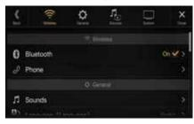
3 Touch the required setting icon on the upper part of the Setup main screen or swipe the list area vertically, then touch the setting item.
