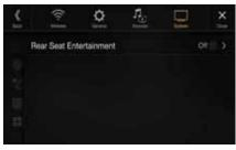
When a Rear monitor equipped with HDMI input is connected to this unit, change this setting to "On." You can output images to the Rear monitor. For details, see "Rear Seat Entertainment Function" (page 18).
