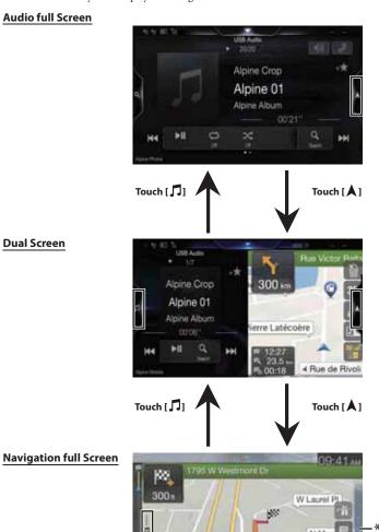
\* Touch [🔍] to switch to the Navigation menu screen. For details of navigation operations, refer to "Navigation System OM" in the CD-ROM.
