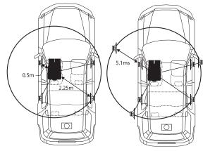
The sound is not balanced because the distance between the listening position and the various speakers is different.
